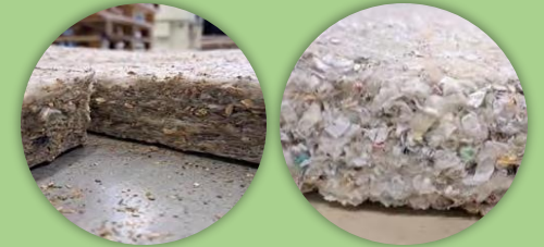
Insulation panels made with green waste (left) and paper waste (right)
