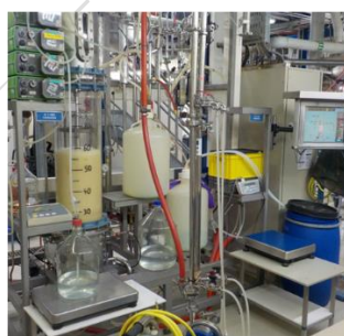
Small Pilot Scale: 50 – 60 L working volume
