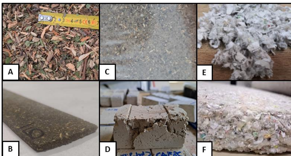
(A) Raw green waste (GW) shredded at 8mm, and (B) panels with GW grinded at 2 mm; (C) Dry organic waste and (D) mortars with it; (E) Paper scraps grinded at 5 mm and (F) thermal insulation panels.
