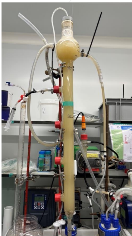
EGSB (expanded granular sludge bed) reactor
